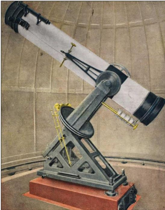
Figure 98: Equatorial Newtonian telescope incorporating a 10-*pouce* Henry-Secretan mirror. Troubetzkoy (1917) says he mounted the mirror himself, and the base is similar to a variable-latitude one invented by him (Troubetzkoy, 1919). However the tube and declination controls show many similarities with Foucault-Secretan instruments (cf. Figures 51 and 82) (after: Troubetzkoy, 1917; courtesy: introni.it).
