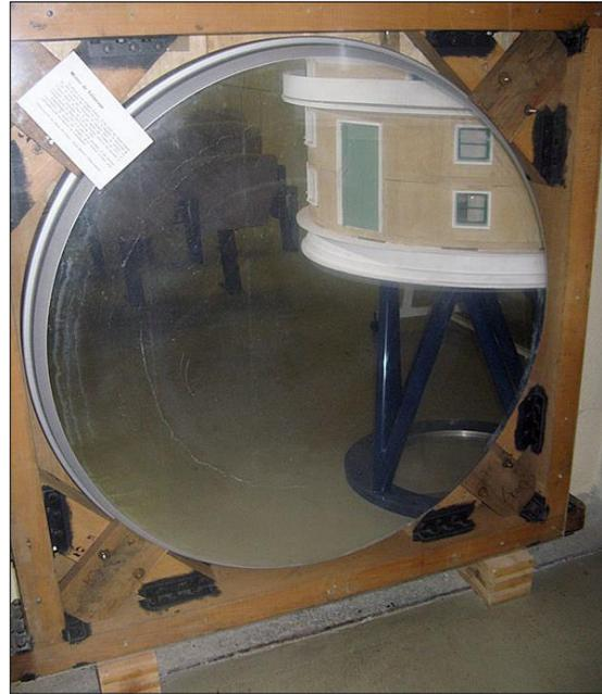
Figure 87: Martin's mirror from the Paris 120-cm telescope was refigured in the 1930s by the optician André Couder and installed in 1942 at the Observatoire de Haute-Provence. The mirror was chipped soon afterwards and is now on display at the Observatory. The damage has been hidden by the large bevel (courtesy: [www.obs-hp.fr](http://www.obs-hp.fr)).
