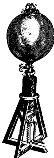
Fig. 3 Piston pump designed by Robert Boyle and built by Robert Hooke in 1658-9.
